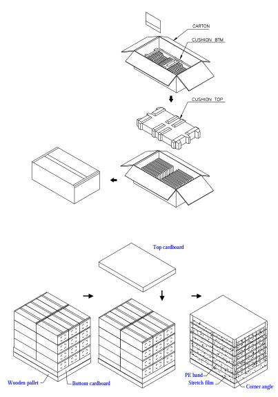
Note : Limit of box palletizing = Max 4 layers(ship and stock conditions)
